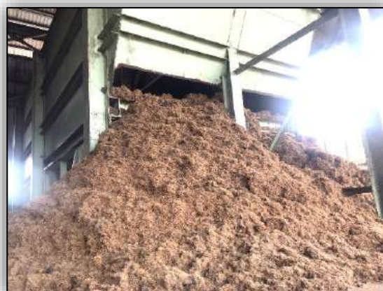
Fiber is stored on-site for use at the mill boiler for steam generation
